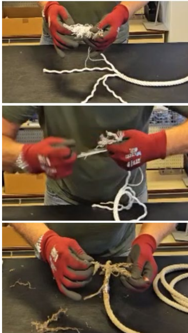
Figure 2: Manual break load test showing (i) (top) a new mainline being separated and braid being exposed; (ii) (middle) a new mainline being put under manual strain, and not breaking; and (iii) (bottom) a worn mainline having been separated and put under manual strain and breaking.
